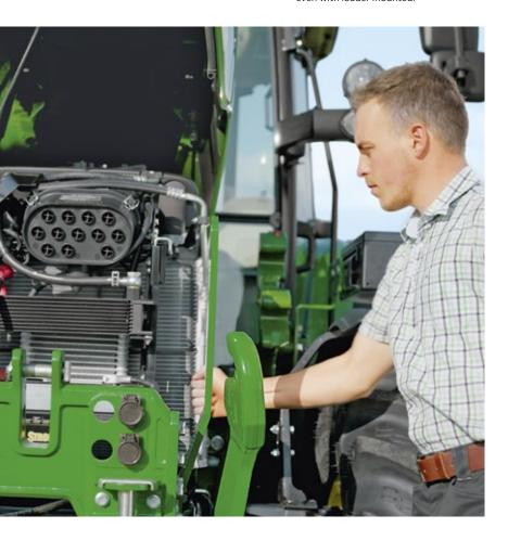
We made all service points accessible from ground level, put sight glasses into most fluid cases, and made sure that you can inspect and change engine air, cab fresh air and recirculation filters without tools. We also put maintenance-free bushings, bearings, and drive shafts wherever possible. So, while there may be no trophy at the end of your day, we promise that your pit stops will be fewer, shorter, and your time in the field longer.
