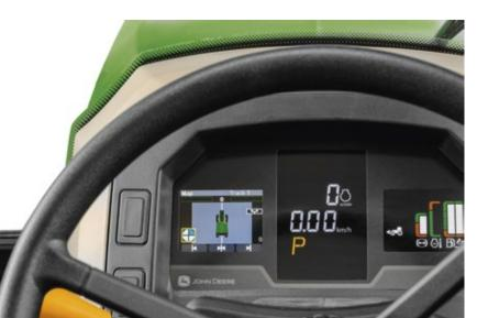
Integrated AutoTrac™ leverages the in-dash display
