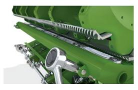
It only takes a few turns with a socket wrench to fully engage the booster bar.
